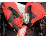
check fluid level monthly. Avoid contact with corrosive deposits and battery acid. Wear eye protection and rubber gloves.
