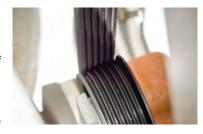
the belt is typically flat and smooth, often rolls against one or more idler pulleys, and may also be used to drive certain components. Most cars use a single serpentine belt for all of the accessories; the belt gets its name from the twisting path it follows to wrap around all the pulleys. However, some cars use additional serpentine or V-belts (see below) to power selected accessories.
