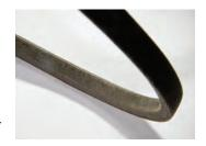
mon on older cars, and are still used today in some applications. Engines equipped with V-belts usually have multiple belts driving the accessories.
