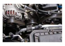
belt tension is with a gauge designed for that purpose, but you can also gauge the tension by applying moderate pressure to the belt at the midpoint of its longest straight section. If the tension is correct, the belt will deflect approximately 1/2 inch.
