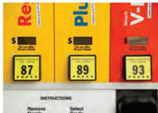
Most cars today are engineered to run on regular grade fuel, though some models with more highly tuned engines call for premium. Modern engines are equipped with knock sensors that allow use of lower grade fuel if the required grade is unavailable. However, engine performance and fuel economy will suffer. Never use less than the recommended fuel grade when the vehicle is heavily loaded or being used for towing.
