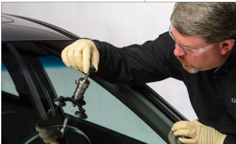
Chip repair can be a cost-effective alternative to windshield replacement.
